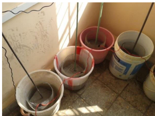
Figure 2: Laboratory set up for Accelerated Corrosion for Epoxy Coated Rebar
